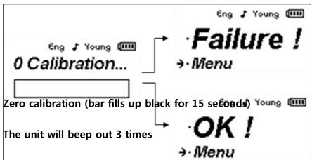
If zero calibration is successful, "OK!" will be displayed. Otherwise, "Failure" will be displayed. (If "Failure" happens see the troubleshooting section)
